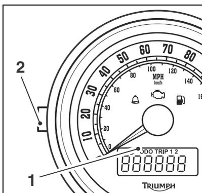
1. Odometer/trip meter/clock display
