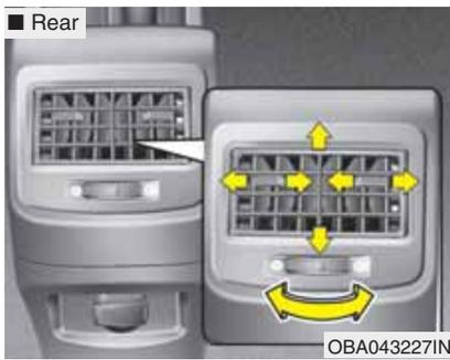
The outlet vents can be opened or closed separately using the thumbwheel. Also, you can adjust the direction of air delivery from these vents using the vent control lever as shown.
