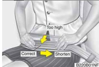
With a 2-point static type seat belt, the length must be adjusted manually so it fits snugly around your hip. Fasten the belt and pull on the loose end to tighten the belt. The belt should be placed as low as possible on your hips, not on your waist. If the belt is too high, it could increase the possibility of injury in an accident.
