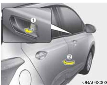
To lock a door without the key, push the inside door lock button (1) to the "Lock" position and close the door (2). (if not equipped with central door lock system)
