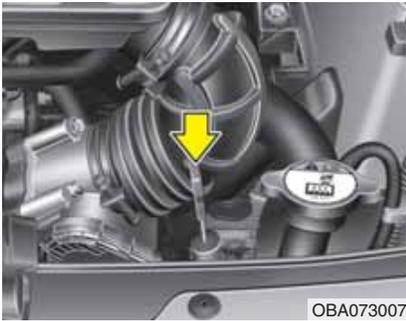
**Checking the automatic transaxle fluid level**
