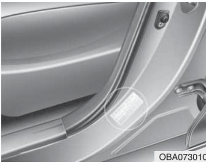
The tires supplied on your new vehicle are chosen to provide the best performance for normal driving. The tire label located on the driver's side center pillar gives the tire pressures recommended for your vehicle.
