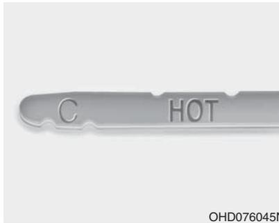
3. Confirm that the fluid level is in "HOT" range on the level gauge. If the fluid level is lower, add the specified fluid in the fill hole. If the fluid level is higher, drain the fluid from the drain hole.
