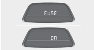
This warning light illuminates if the fuse switch in the fuse box is OFF. Turn the fuse switch on, when the "FUSE ON" warning light illuminates.
