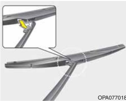
3. Install the new blade assembly by inserting the center part into the slot in the wiper arm until it clicks into place.
