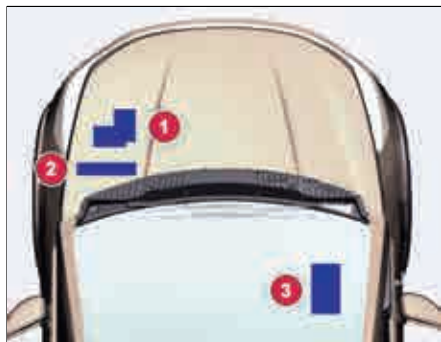
Fuse location- Engine and battery
