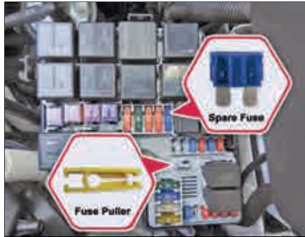
Engine compartment fuse box
