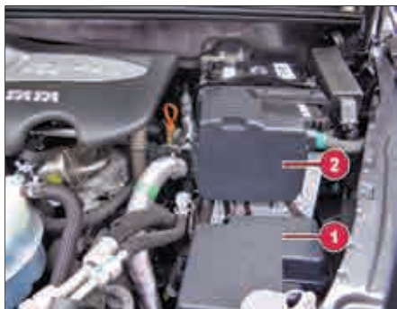
Fuse location- Engine and battery
