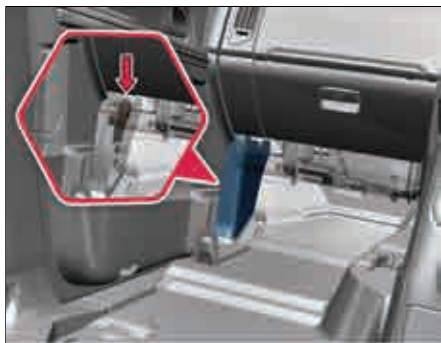
Inertia switch location
