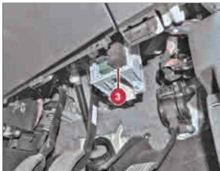
Fuse location- Cabin compartment
