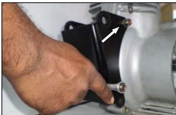
☆ Remove Mudguard mounting clip & Rear Engine Mounting Bracket.
