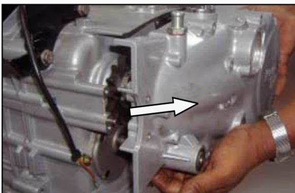
**NOTE :** Remove the stator coupler from the wiring harness before removing RH Cover.
