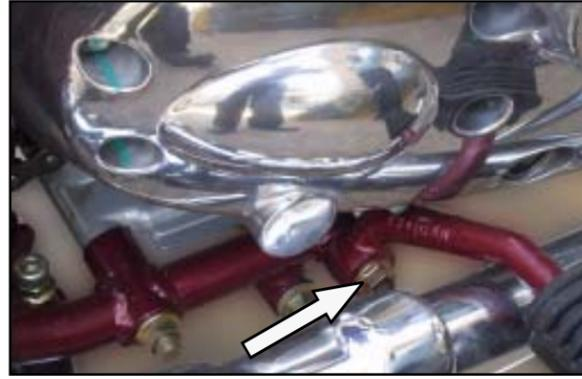
**NOTE :** Ensure step face of jack shaft gear should face inside (Towards Crank case LH)
