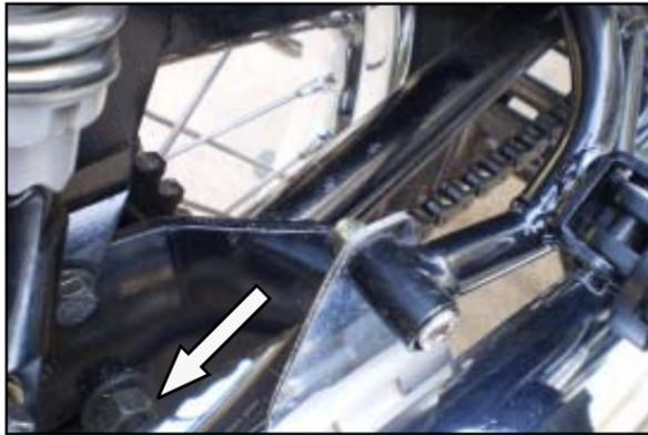
**NOTE :** Loosen the rear brake rod adjuster nut so that the brake pedal can be depressed to allow the exhaust pipe to be removed.
