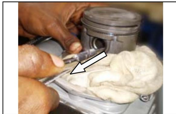
**NOTE :** Carefully remove the piston pin clip from the piston while covering Crank case neck with a shop towel, as shown.
