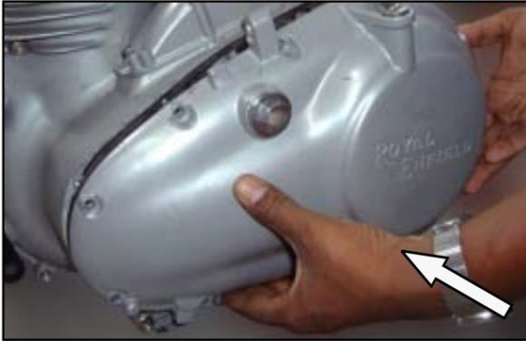
**NOTE :** Ensure 2 Nos. dowel pins are located properly. Apply LOCKTITE 5699 RTV silicon liquid gasket.
