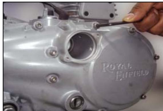
**NOTE :** Use special tool No. ST 25592-4 to lock connecting rod movement during tightening magneto nut.
