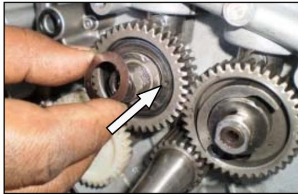
**NOTE :** To reduce axial play in between Cam Gears outer surface and steady late, additional shim may be added as per need.
