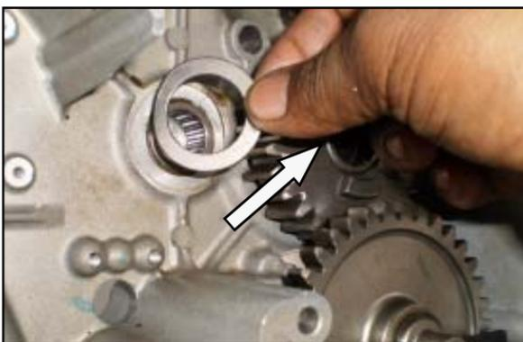
**NOTE :** Ensure special thrust washer profile is facing towards sleeve gear.
