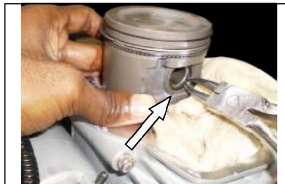
**NOTE :** Carefully fix the piston pin clip into the piston boss while covering Crank case neck by shop towel / chamois cloth as shown in Fig.
