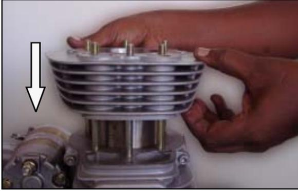
**NOTE :** Do not use any sharp objects to press piston rings against groove. Use thumb finger force to locate rings in its position properly.
