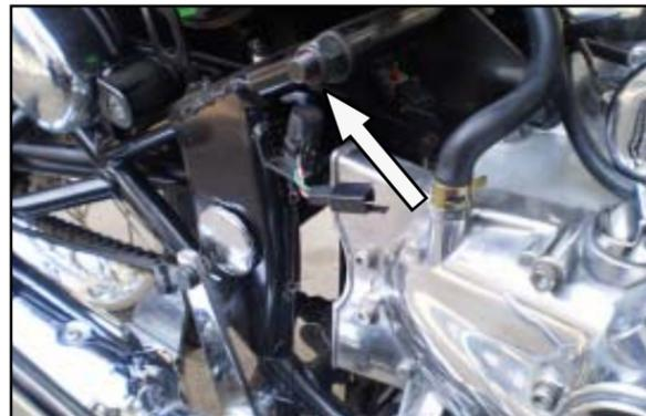
☆ Remove the front engine mounting nut
