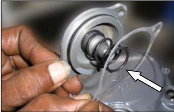
**CAUTION :** Care must be taken while fixing cover due to spring force and gasket.
