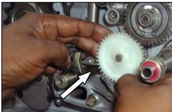
**NOTE :** Ensure the short boss of the gear is facing outwards.
