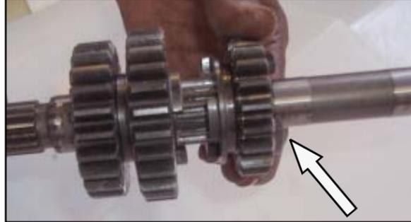
**NOTE :** Ensure 2nd gear selector fork groove side is facing towards MS 4th gear.
