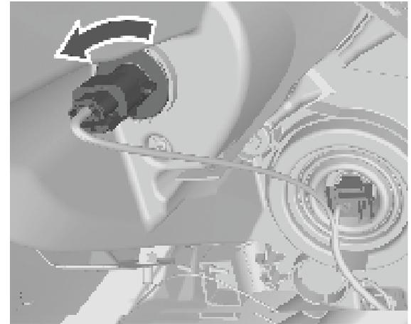
1. Rotate bulb holder anti-clockwise and disengage.
