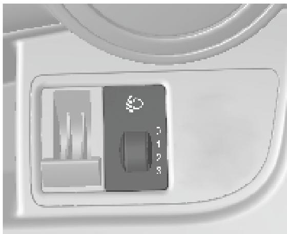
To adapt headlamp range to the vehicle load to prevent dazzling: turn knob to required position.
