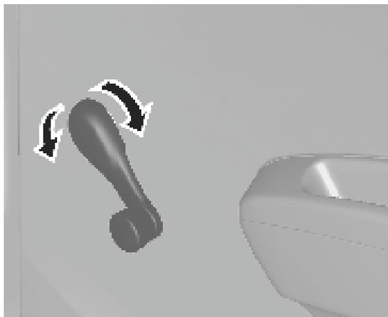
The door windows can be opened or closed with the window winders.
