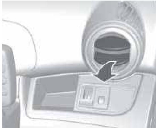
Press the cover of each vent to open the side vents, and rotate it to the direction you want.
