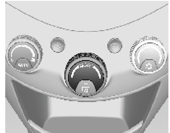
Turn the MODE knob once or more for desired adjustment. The air distribution is indicated on the display.
