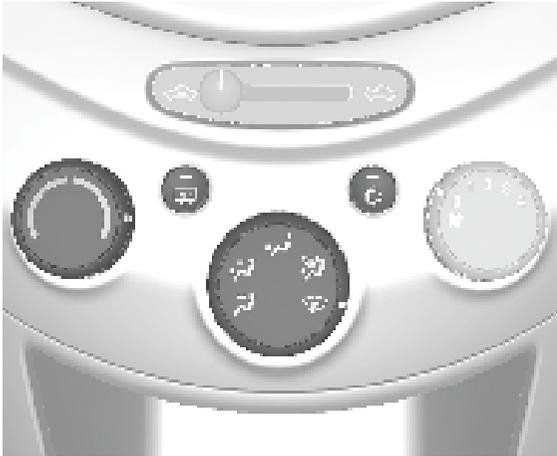
1. Set the recirculation mode to outside air mode and turn the air distribution knob to DEFROST
