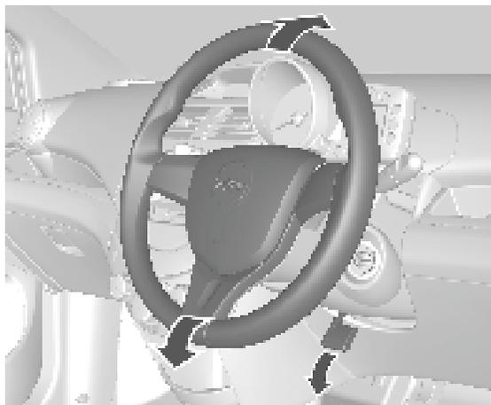
Unlock lever, adjust steering wheel, then engage lever and ensure it is fully locked. Do not adjust steering wheel unless vehicle is stationary.
