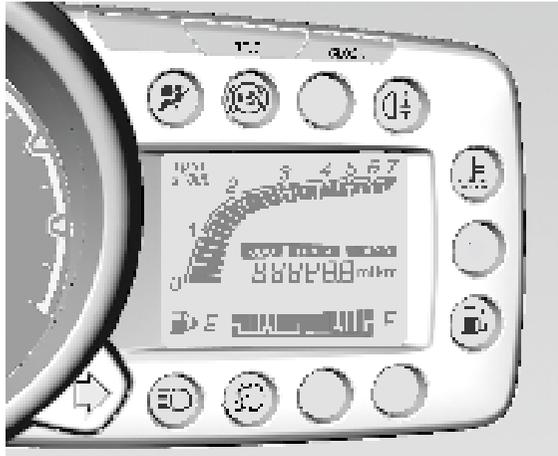
Trip computer provides the driver with driving information such as driving distance.
