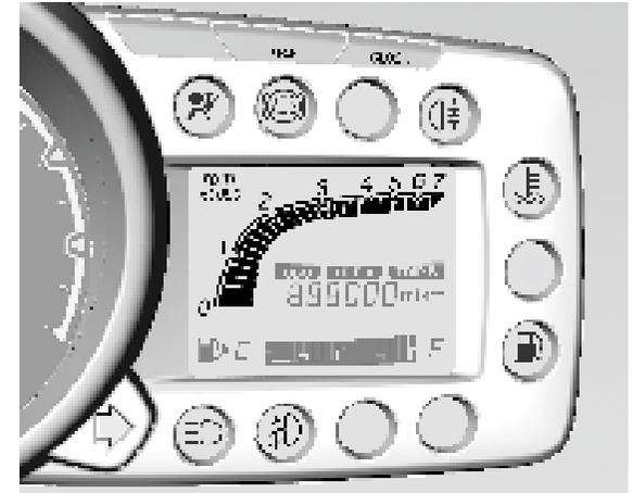
Displays the engine revolutions per minute.
