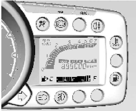
Displays the fuel level in the tank.
