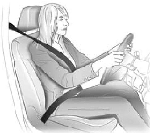
The belts are locked during heavy acceleration or deceleration of the vehicle for the safety of the occupants.
