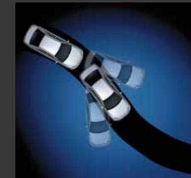
**Vehicle Stability Control:** Be in control at every turn. The VSC applies an active braking force independently to the four wheels and ensures stability during turnings.
