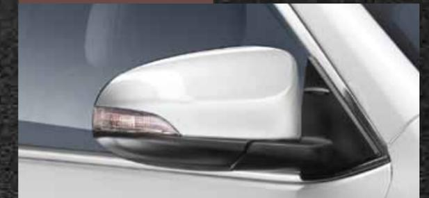
**Auto Folding & Reverse Linked ORVMs with Memory:** A unique feature that stores the previous position of the side view mirror and automatically tilts to assist while reversing.
