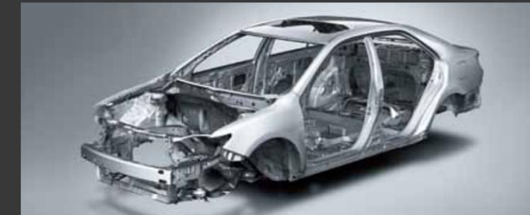
**Impact Absorbing Vehicle Body:** Sturdy from every side. The body structure of the all New Camry Hybrid is constructed in a way that it disperses collision energy through many frame components for effective energy absorption. Making it safer during accidents.
