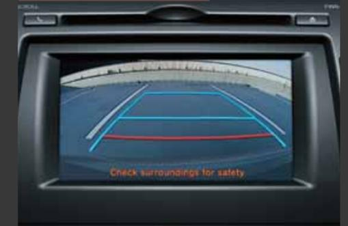
**Back Monitor with Corner Sensors:** Senses what's around and what's behind. The rear camera displays a clear view of the rear while the corner sensors notify the driver of any obstacle near the corner bumpers.
